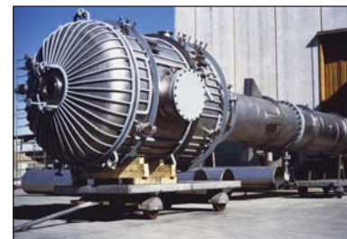
Colonna di stripping in Titanio Gr.2 Stripping column in Titanium Gr.2
