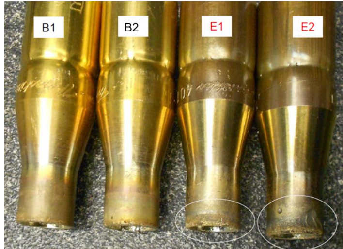
Picture 19: Gas nozzles made from leaded brass (B1 and B2) compared to such made from silicon brass (E1 and E2). The front end of C69300 nozzles (E1 and E2) melted during the test.
