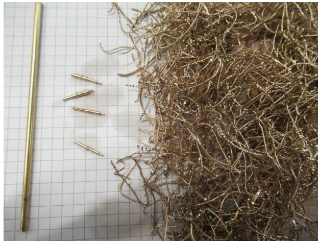
Picture 21: Chips resulting from turning contacts.
