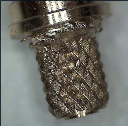
Picture 14: A knurl made from CuZn42 with sharp edges and broken material.
