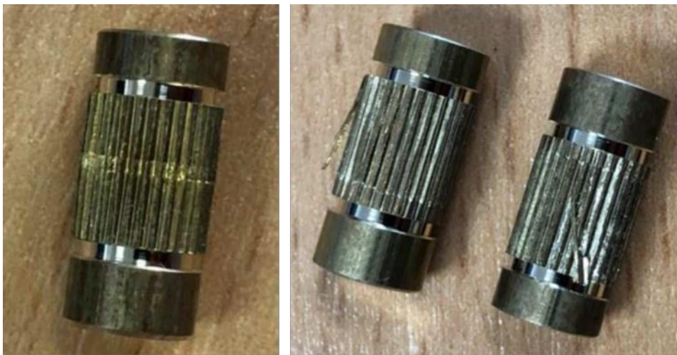
Picture 18: A knurl pressed from CuZn39Pb3 (left) and two knurls pressed in CuZn21Si3P with loose particles (right).
